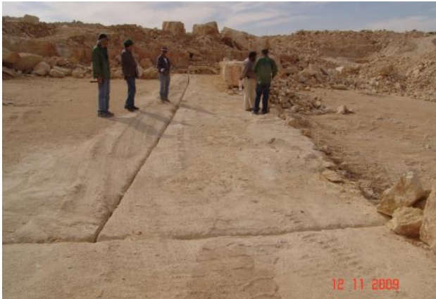
E. Trenches of the disc saw immediately prior to rock extraction (AE)
