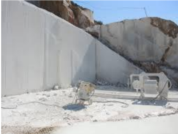
A. Diamond wire saw (type 1)
