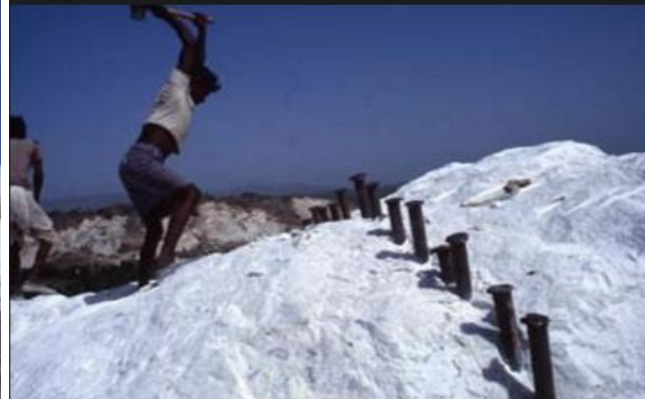
B. Placing long chisels into the drilling holes. Hammering on the chisels till the block is separated from the natural formation
