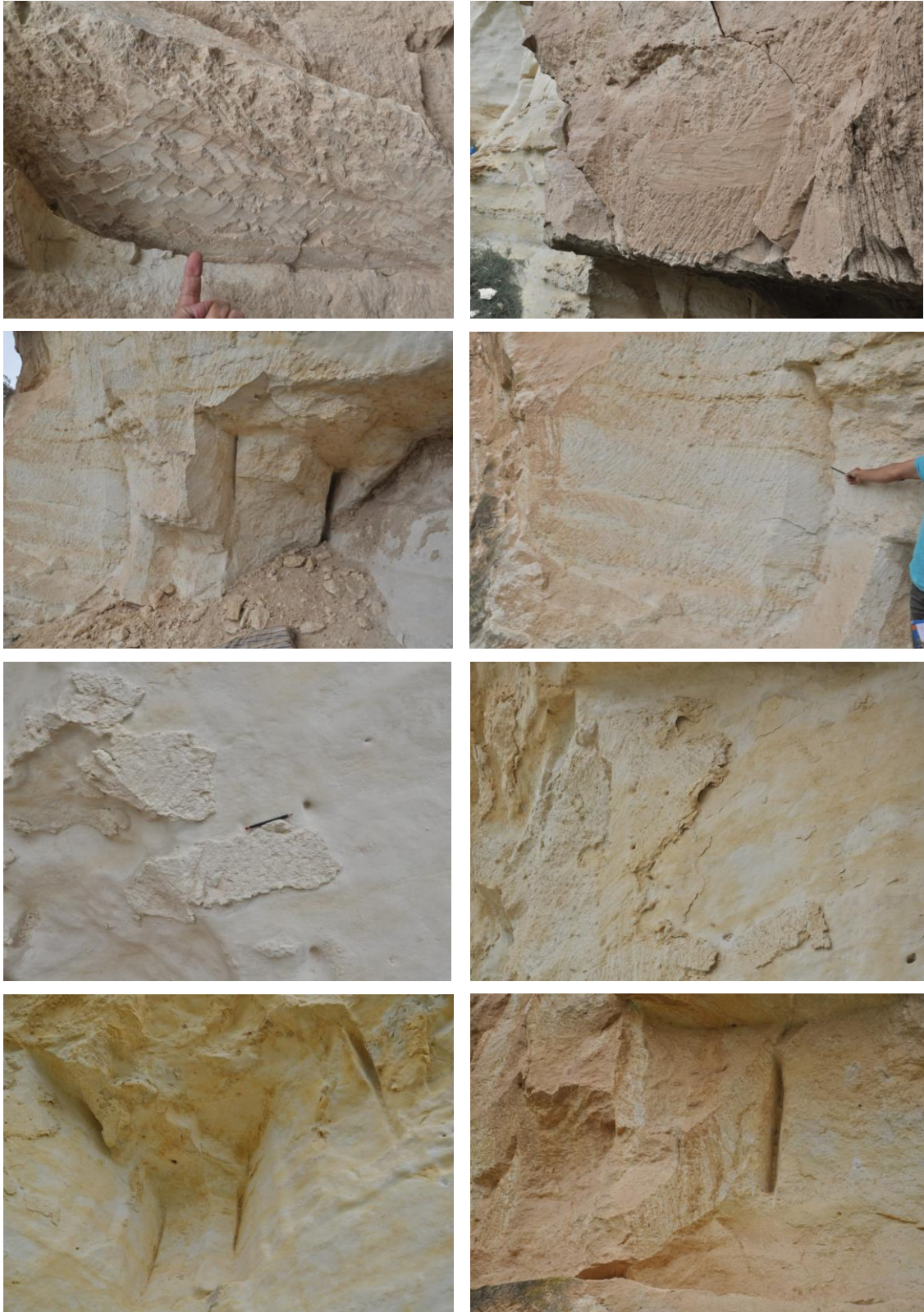
Figure 28b: Imprints of the mining tools
