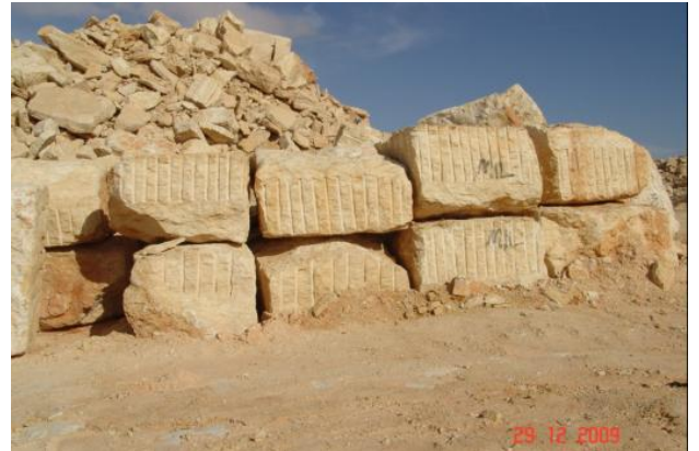
D. Storing blocks in the quarry until shipping to the sawmill (AE)
